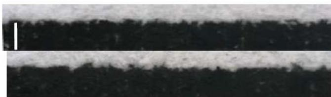
*Figure 5. Micrograph of printed lines with different line acuity. Top: 10 um raggedness. Bottom: 15 um raggedness. Length of measurement bar is 0.5 mm*
